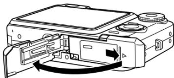
2. While pulling the stopper in the direction indicated by the arrow in the illustration, align the arrow mark on the battery with the arrow mark on the camera and slide the battery into the camera.
